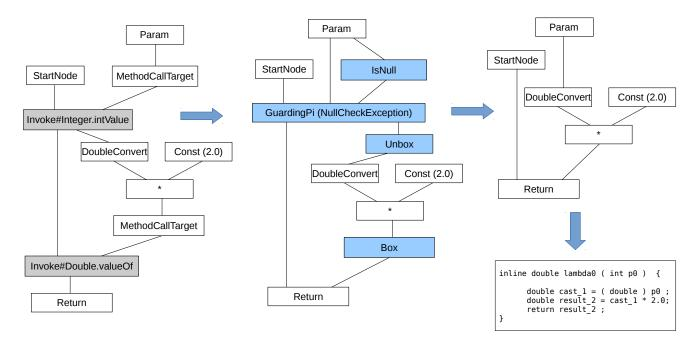
Figure 4: Graal IR optimisation phases and C OpenCL code generation. The left side shows the Graal IR for the input code in Java (lambda expression). Then, in-line Graal IR optimisation is invoked and it produces the second graph. As we produce C OpenCL code, we do not need to support null pointers, box and unbox, therefore this graph is optimised given the graph in the right side.
