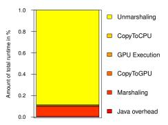
Figure 5: Breakdown of the total runtime of the Black Scholes application into single steps. The marshalling and unmarshalling steps are constituting over half of the total runtime.
