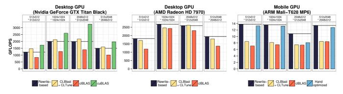
**Figure 7:** Performance of matrix multiplication on two desktop GPUs and one mobile GPU for different input sizes. The *rewrite-based* approach is the only one that achieves performance portability across desktop-class *and* mobile GPUs.
