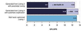
**Figure 6:** Performance of different matrix multiplication kernels. Our fully automated exploration technique produces a kernel that outperforms the manually optimized kernel.
