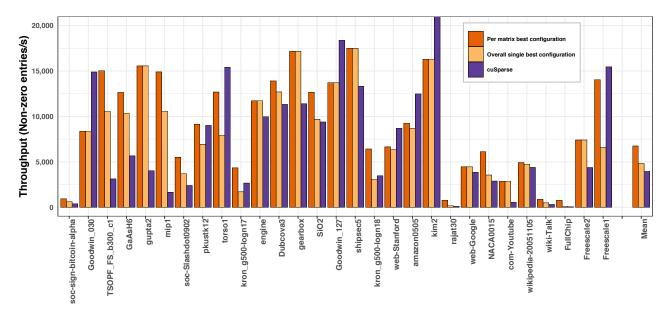
Figure 8. Comparison of the throughput of various configuration vs cuSparse, in input matrix elements read per second
